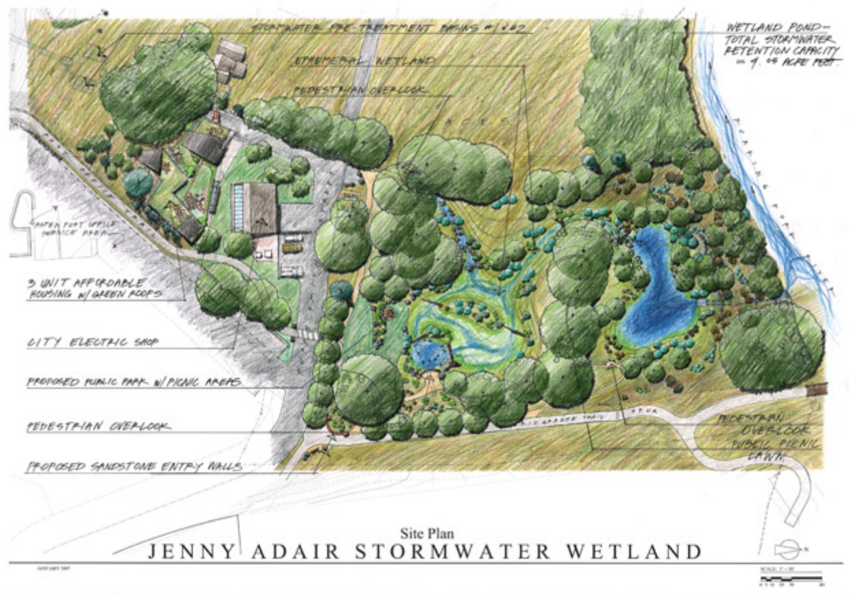
Figure 3: Jennie Adair Regional Stormwater Quality Project – “A constructed wetlands basin is a shallow retention pond that has a continuous base flow which promotes the growth of rushes, willows, cattails and reeds. The shallow pond, along with vegetation, slows down runoff and allows time for sedimentation, filtering, and biological uptake. Wetlands greatly improve water quality while at the same time providing natural aesthetic areas, increasing wildlife habitat, and providing erosion control. Constructed wetlands are engineered to mimic natural wetlands which can be viewed as the “kidneys” of the hydrologic cycle due to their filtering and cleansing capabilities. 2 ” These important areas in Aspen are both innovative and critical. These areas of green infrastructure treat urban runoff creating better conditions for the rest of the riparian area which maintain aesthetic, habitat and cultural values.
