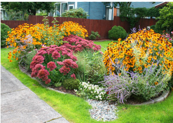
Figure 8.47 Rain gardens are used to collect and filter stormwater runoff. As seen in the examples above they can be planted in a variety of areas with a wide variety of plant life from flowers and grasses to trees.
