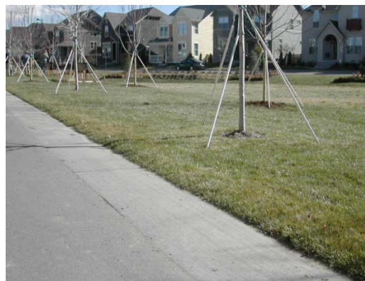
Figure 8.22 A curbless street allows parking lot stormwater to flow evenly from the road through a grass buffer.
