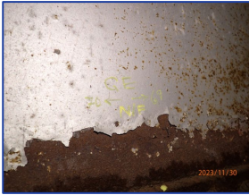
Failure of protective coating
